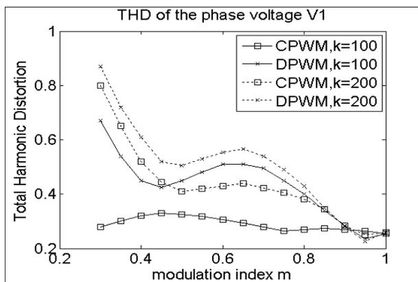
Figure 20.  $THD$  factor of the phase voltage  $V_I$  versus modulation index  $m_H=m_L$ . ( $F=50\text{Hz}$ ,  $F_s=1.35\text{kHz}$ ,  $V_H=V_L$ ) [14].
