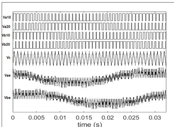
So, modified schemes of synchronous PWM, elaborated for adjustment of five-phase dual-inverter system with open-end winding of induction machine, provide symmetry of the phase voltage during the whole control diapason, including the zone of overmodulation [9; 16]. Spectra of the phase voltage of five-phase systems with schemes of synchronous PWM do not contain even harmonic components and subharmonics, which is especially important for installations with an increased power level.
