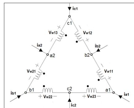
**Figure 7.** Stator windings of double-delta-sourced winding drive system [18].
