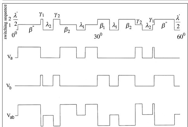
**Figure 1.** Switching state sequence, phase voltages  $V_a$ ,  $V_b$ , and line voltage  $V_{ab}$  of three-phase inverter with synchronous multi-zone modulation for the 60°-clock-cycle [6].
