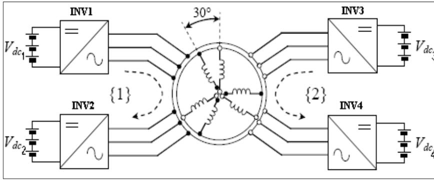
**Figure 10.** Topology of six-phase system on the base of four inverters (the first inverter group INV1+INV2, and the second inverter group INV3+ INV4) supplying open-end windings of asymmetrical six-phase induction motor with two sets of winding spatially shifted by 30 el. degrees [12].
