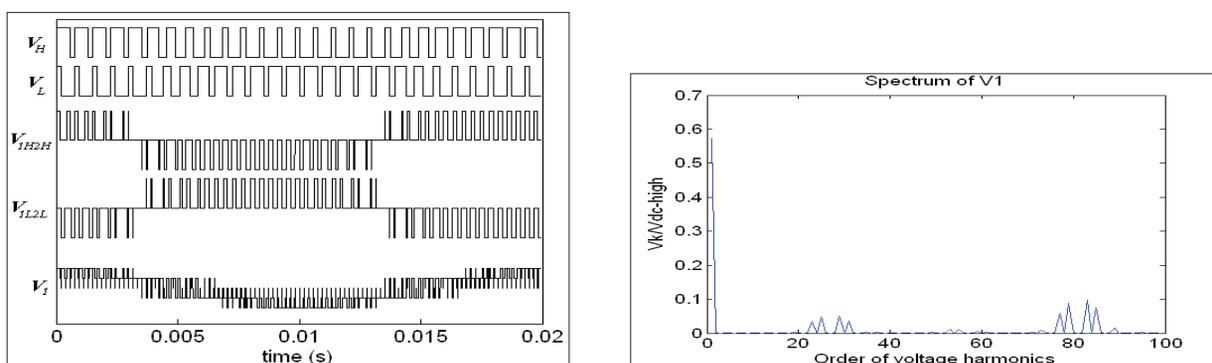
Figure 19. Pole voltages  $V_{IH}$  and  $V_{IL}$ , line voltages  $V_{IH2H}$  and  $V_{IL2L}$ , and phase voltage  $V_I$  (with its spectrum) of PV system with continuous synchronous PWM ( $F=50\text{Hz}$ ,  $F_s=1.35\text{kHz}$ ,  $V_H=V_L$ ,  $m_H=m_L=0.45$ ) [14].
