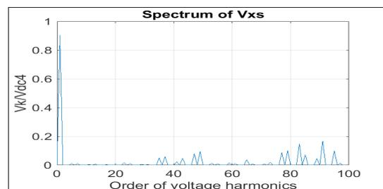
**Figure 12.** Spectra of the phase voltages of the balanced six-phase system [12].
