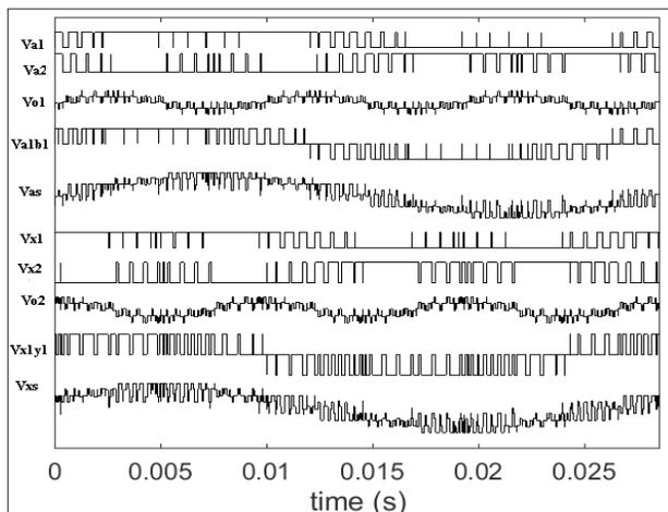
**Figure 11.** Basic voltage waveforms of six-phase system with synchronous discontinuous PWM ( $P_1=0.23, P_2=0.27, P_3=0.24, P_4=0.26, V_{dc1}=0.75V_{dc4}, V_{dc2}=0.9V_{dc4}, V_{dc3}=0.8V_{dc4}, V_{dc4}=1, m_1=0.93, m_2=0.78, m_3=0.87, m_4=0.7$ ) [12].
